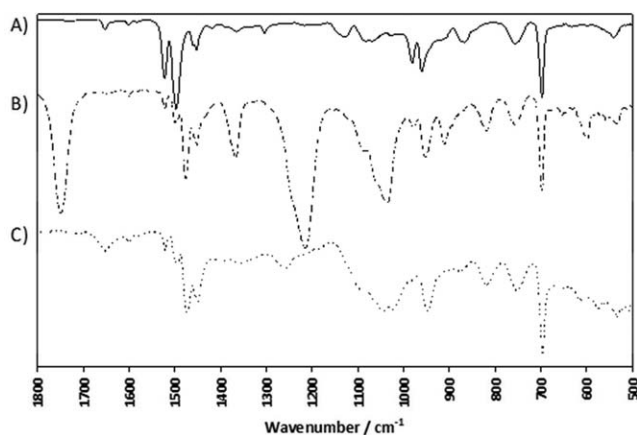
Figure 7. IR spectra of BF films of PS- b -PFS (A), PS- b -PFS-GlcAc4 (B), and PS- b -PFS-GlcOH (C).
